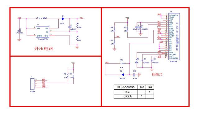
The I2C communication interface consists of slave address bit DC, I2C-bus data signal SDA (SDAOUT/D2 for output and SDAIN/D1 for input) and I2C-bus clock signal SCL (D0). Both the data and clock signals must be connected to pull-up resistors.
